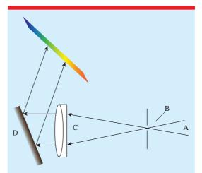
**Figure 2.** Diagram of the Littrow spectroscope. The solar light rays travel from telescope A (Newtonian 200 mm, f/10) to slit B, collimator lens C (achromatic doublet, 800 mm focal length), diffraction grating D (50 mm  $\times$  50 mm, 1200 l/mm), and to the projected solar spectrum E (30 cm in length).
