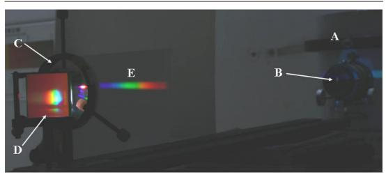
**Figure 3.** Image of the Littrow spectroscope used in the *Solar Physics* course. A is the telescope, B is the slit, C is the collimator lens, D is the diffraction grating and E is the projected solar spectrum.
