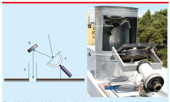
**Figure 1.** Left: diagram of a heliostat with movable primary mirror (A), fixed secondary mirror (B) and telescope (C). Right: image of the heliostat, where A is the primary mirror and B is the secondary mirror.
