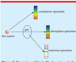
**Figure 5.** Illustration of Kirchoff's three laws. At the top, a continuous spectrum is produced, for example, by using an incandescent lamp. In the middle is an absorption spectrum, like the solar visible spectrum. At the bottom is an emission spectrum produced by a spectral lamp.
